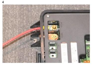
Connect Positive Lead – Connect the 10 gauge positive (red) lead to the positive post on the power module as shown.
