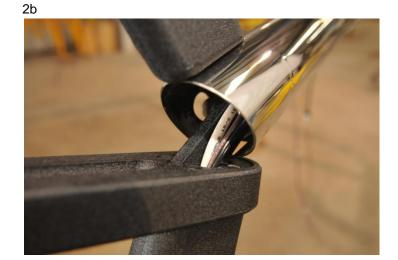
Run wires through Tower Base -Run the remaining two light wire leads down through the Tower Base alongside the all-around light wire. Once the wires have been run through the base, raise the tower.
