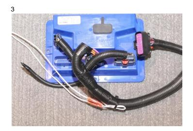
Connect Leads to Computer – Locate the instrumentation computer, then locate the two leads – one solid white and one white with black stripe – that exit the harness about 6" from the computer. Connect the solid white lead and the white lead with the black stripe at the computer to the solid white lead and the white lead with the black stripe coming from the relays.
