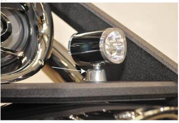
Aim Light Assembly -Loosen the Set Screw in the Base, point the Light in the desired direction, and then re-tighten the Set Screw.
