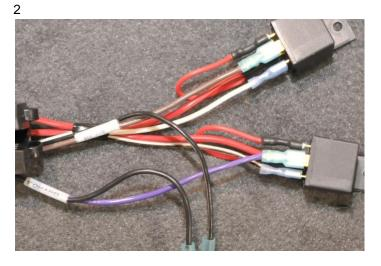
Crimp Positive Leads – Crimp female spade terminals to the positive leads (brown and purple) coming forward from the tower. Connect the purple lead (forward tower circuit) to the relay that has the white lead with black stripe (forward dash circuit) as shown. Connect the brown lead (rear tower circuit) to the relay that has the solid white lead (rear dash circuit) as shown.
