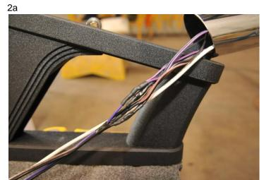
Pull the wires until the port/starboard splice is inside the tower and above the heim joint, as the splice is too large to pass through the Tower Base.
