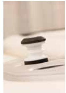
Figure 2-14. Pivoting-head Ski Pylon
