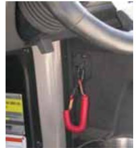
Figure 2-8. Emergency Engine Stop Switch
