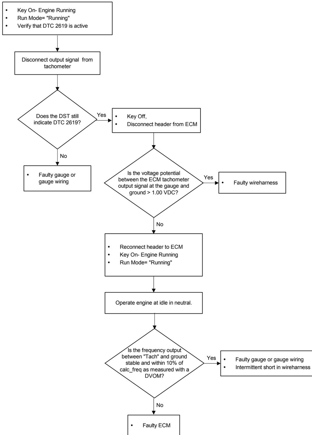
$$\text{calc\_freq (hz.)} = \frac{\# \text{ of cyl}}{2} \times \frac{N}{60}, \text{ where } N = \text{engine speed in RPM}$$
