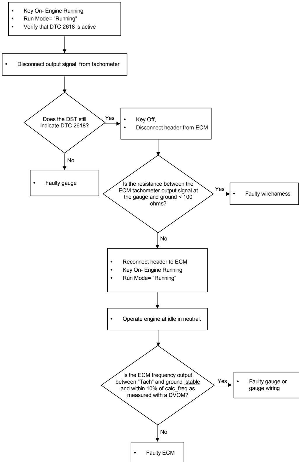
$$\text{calc\_freq (hz.)} = \frac{\# \text{ of cyl}}{2} \times \frac{N}{60}, \text{ where } N = \text{engine speed in RPM}$$
